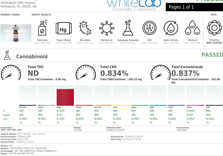
Full Spectrum cannabinoid analysis utilizing High Performance Liquid Chromatography with UV detection in accordance with E.S. Rule 64ER20-39
